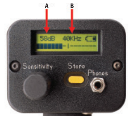
FIGURE 11. Shown here is a dial reading of a typical ultrasound unit
