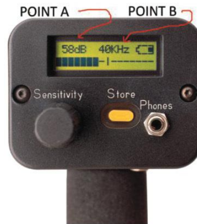
Figure 2: High Frequency Ultrasound Unit Information; "A" is the dB reading and "B" is the KHz setting.
