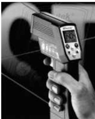
**Figure 9. Infrared temperature gun.**
