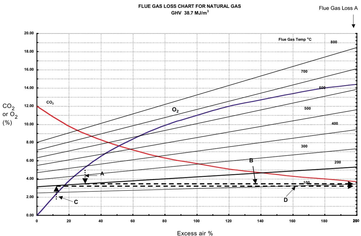
Figure 1: Flue gas loss charts for natural gas
