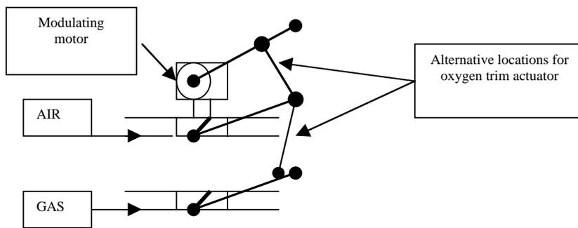
Figure 2: Linked valve air–gas ratio control
