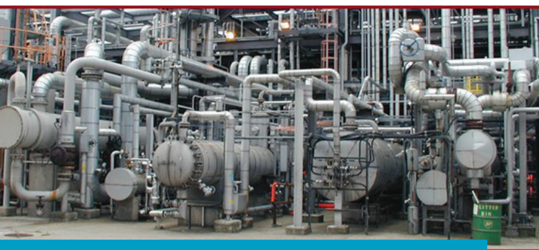
Figure 2. Heat Exchangers in a Process Plant
