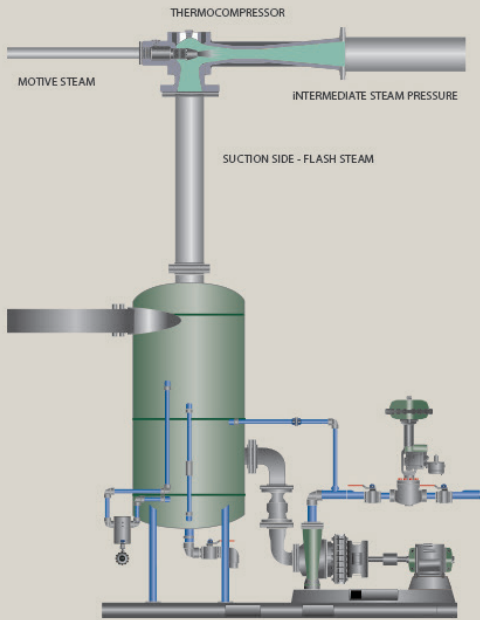
Figure 3: Thermocompressor off a Flash Tank Arrangement
